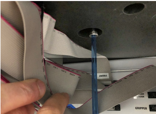
Figure 20 Drainpipe attachment to the cooling unit enclosure
