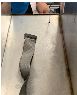
Figure 8 Aligning enclosure box mounting holes
