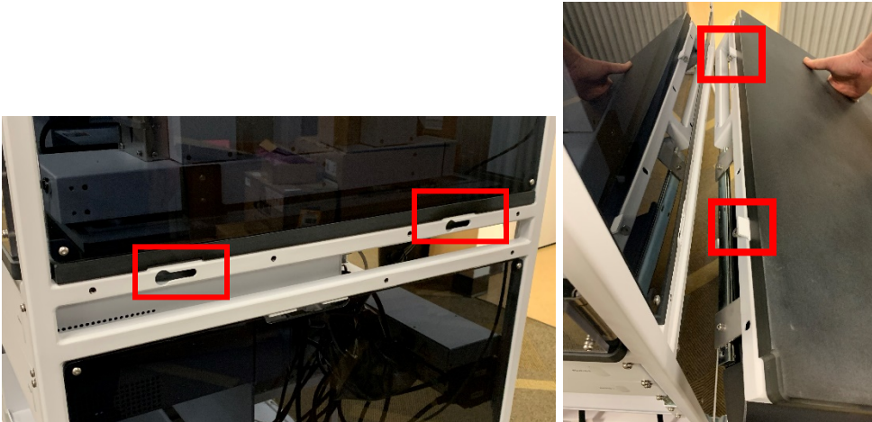
Figure 1 Placing overhang bolts into the frame
