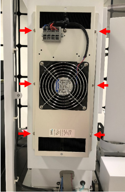
Figure 21 Attachment points for TEC unit
